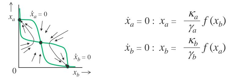
System is **bistable**: two stable and one unstable steady state.
